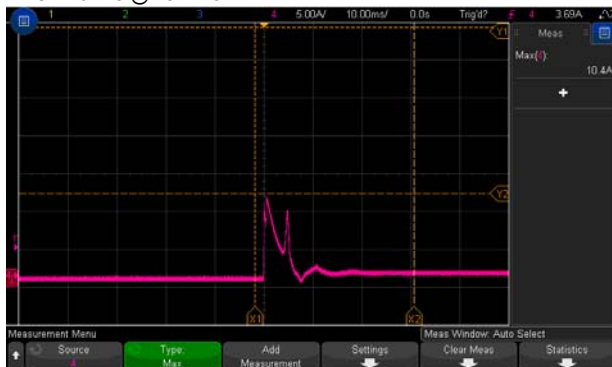
INPUT=48VDC @ FULL LOAD
