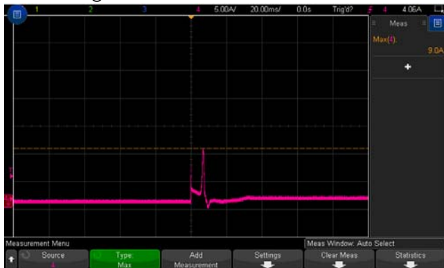
INPUT=24VDC @ FULL LOAD
