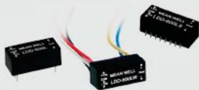
▲ LDD-300~700L/W/LS L/LW: 22.6x 9.9x 8.9 mm LS: 25.4x 10.5x 9.3 mm
